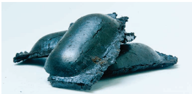
ABOVE - A view of the larger fuel pieces made in the newly-acquired pelletizing machine at NRRI's COLERAINE ENERGY LAB.
