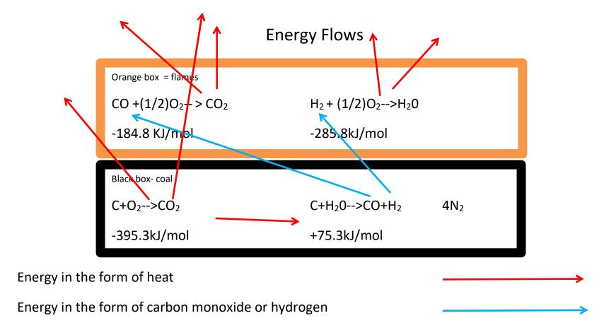
The temperature of the firebed depends on difference between the heat produced by combustion, and the heat absorbed by gas production.
