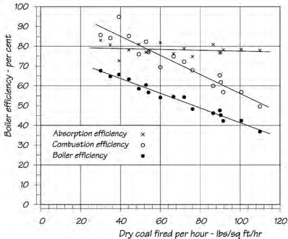
Fig. II.4 – Boiler efficiency curves for Pennsylvania Railroad E2a 4-4-2 N° 5266 tested at Altoona in 1905 – analysis by Lawford Fry
