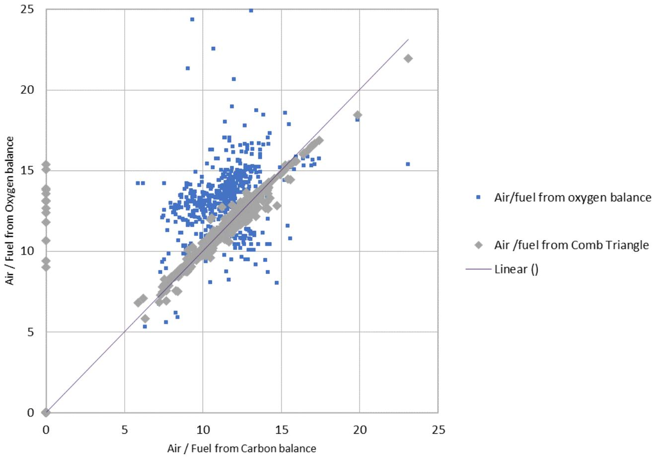
**Figure 5: Comparison of air to fuel ratio derived from carbon balance, oxygen balance and combustion triangle method.**
