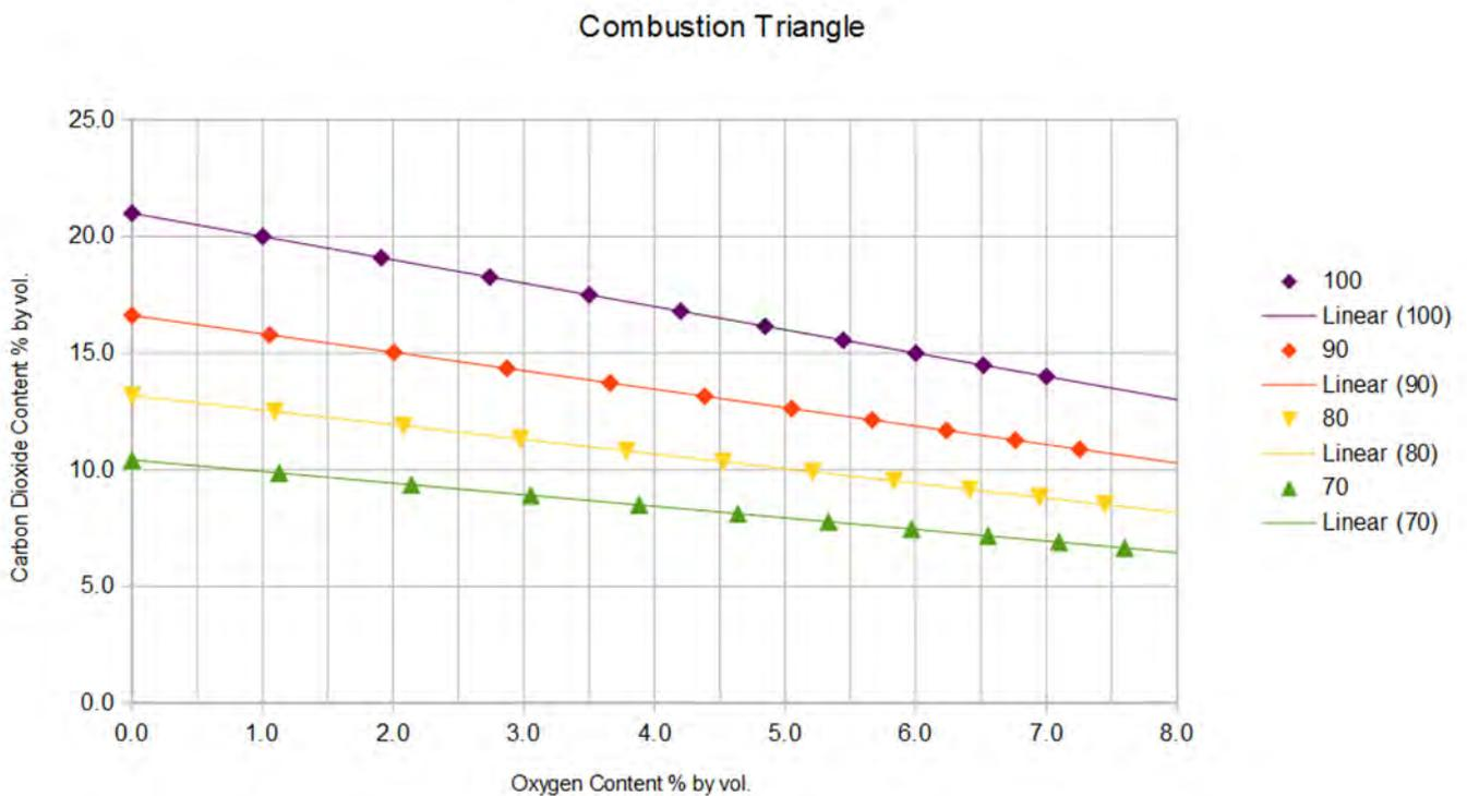
**Figure 2: Combustion triangle drawn for four hydrocarbon fuels.**
