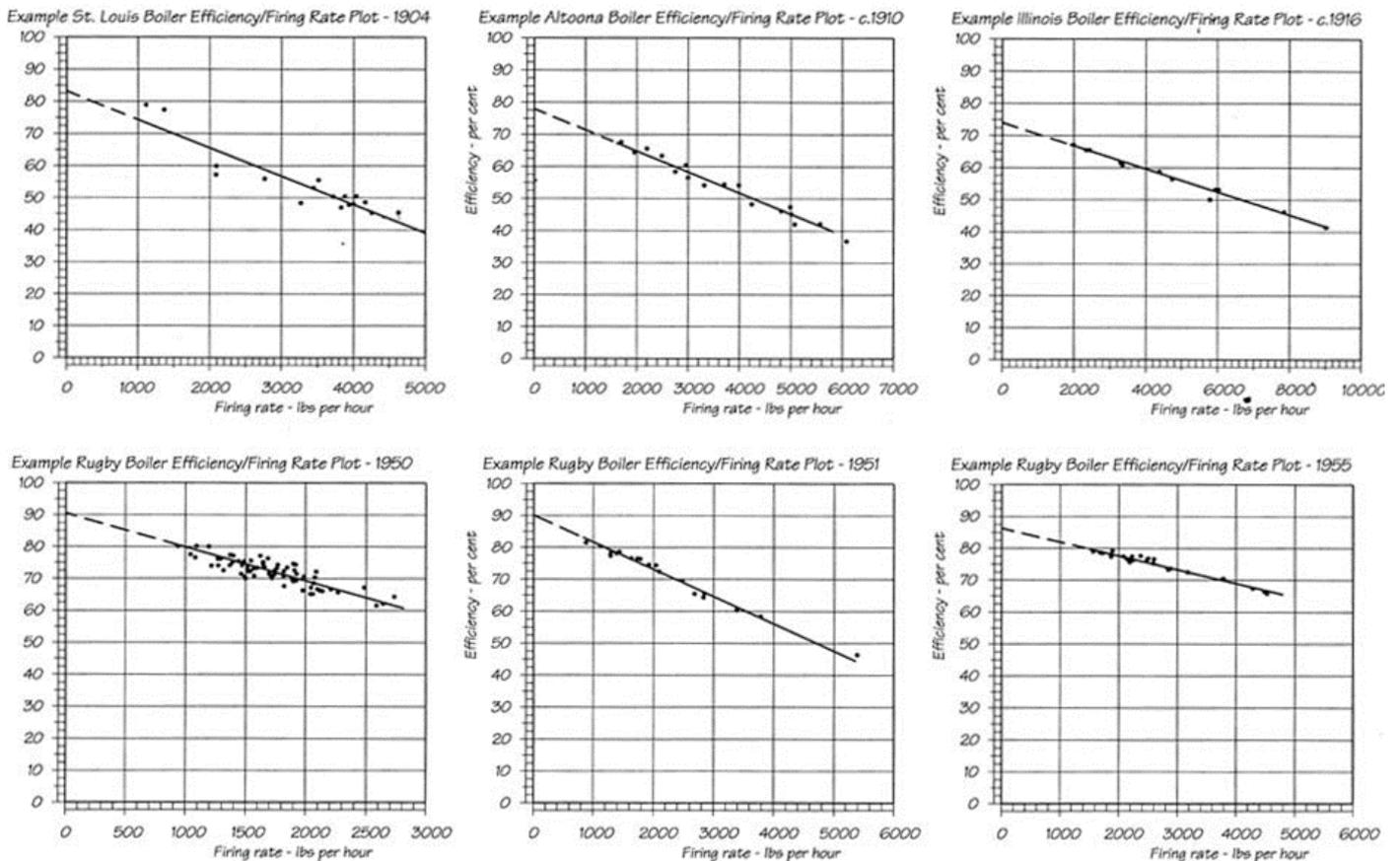
**Fig. II.5 - The improvement in the accuracy of boiler efficiency tests with experience**
