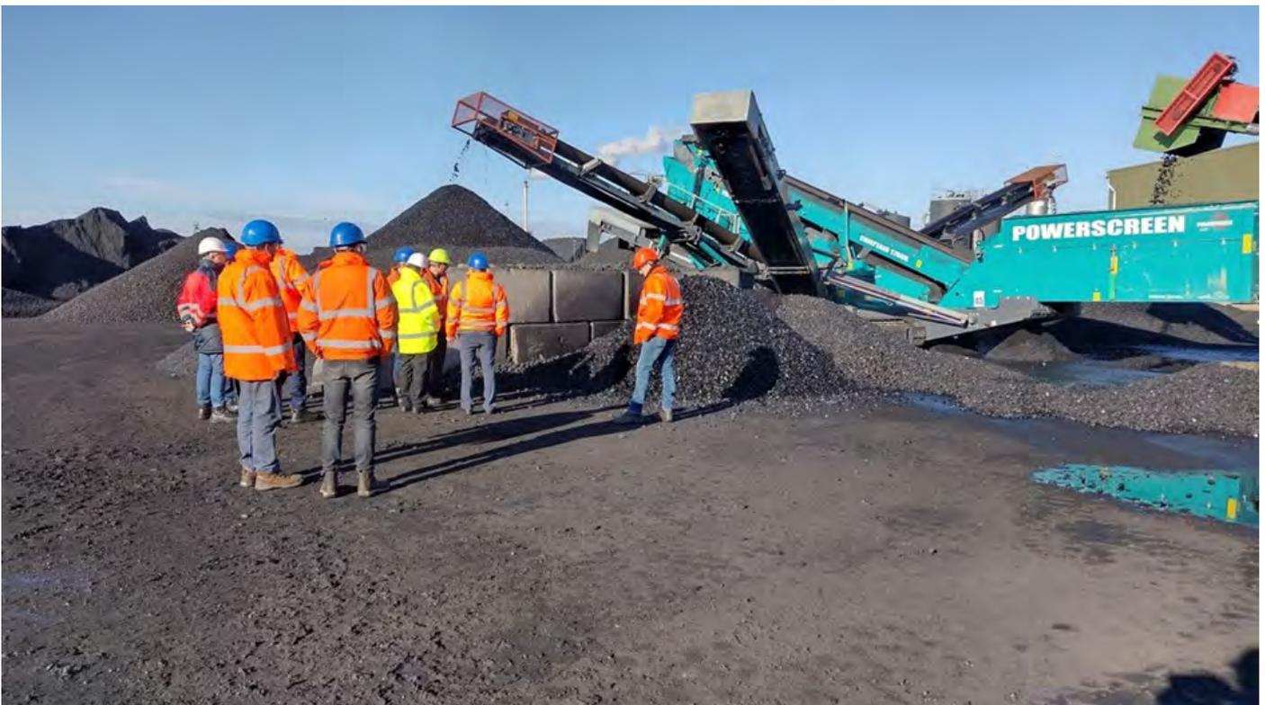
**Screening Plant to sort coal into different sizes**
