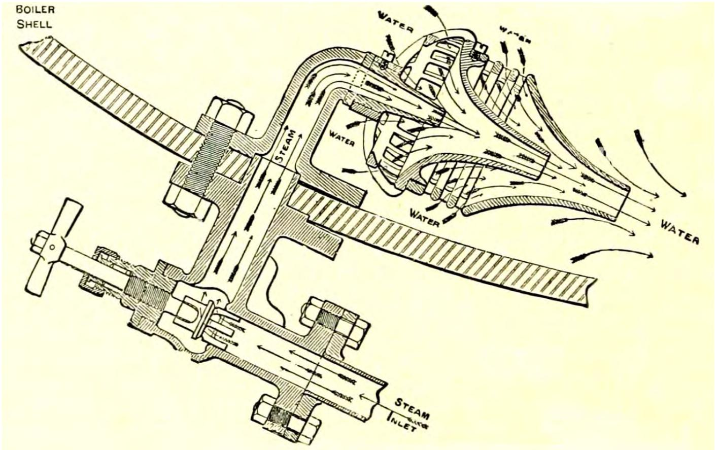
*Hydrokineter in close up (above), and attached to the boiler (below)*
