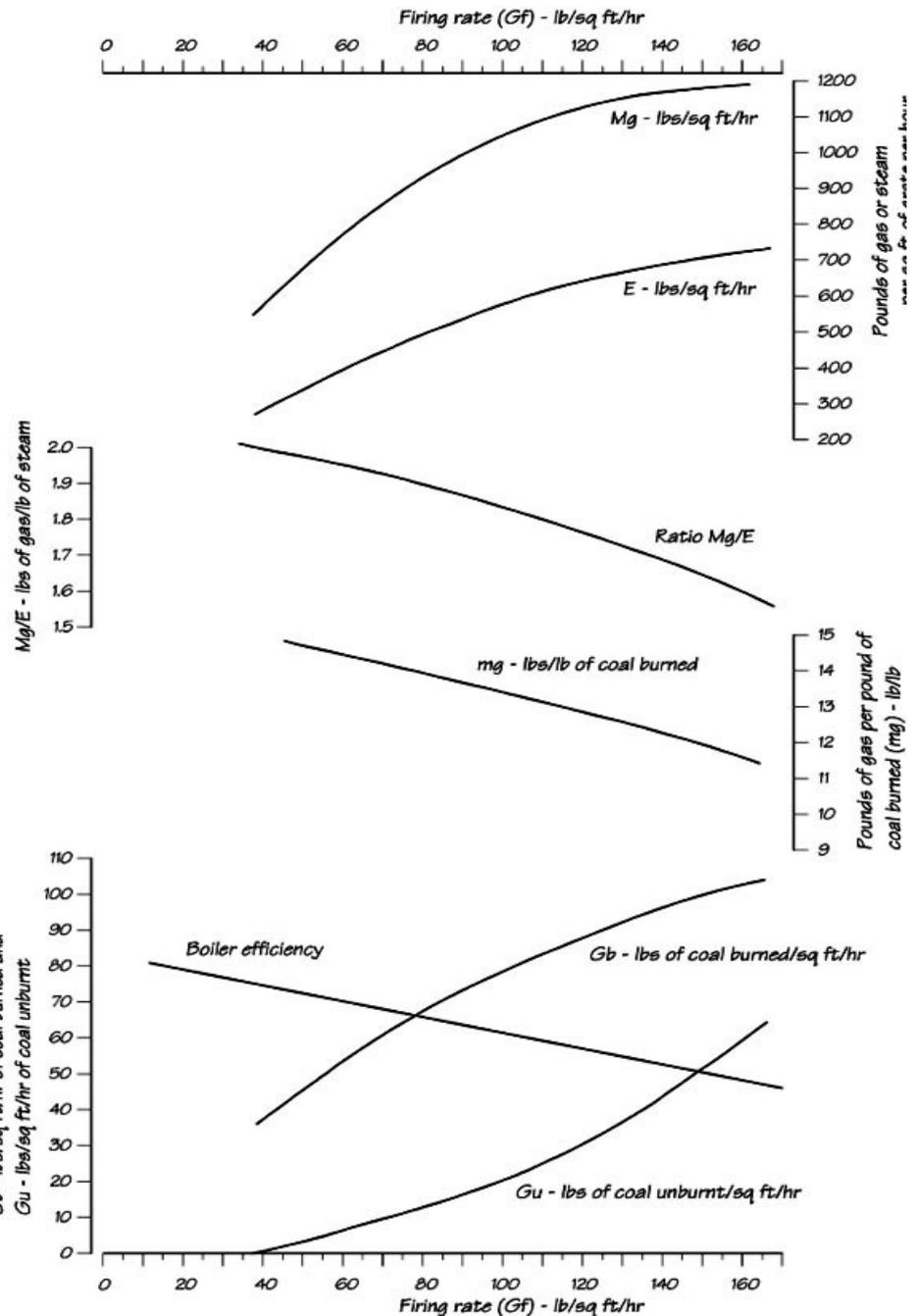
Fig IV.24 - Boiler performance chart for unidentified SAR locomotive - Dr M M Loubser's paper "Some Aspects of Railway Mechanical Engineering"
