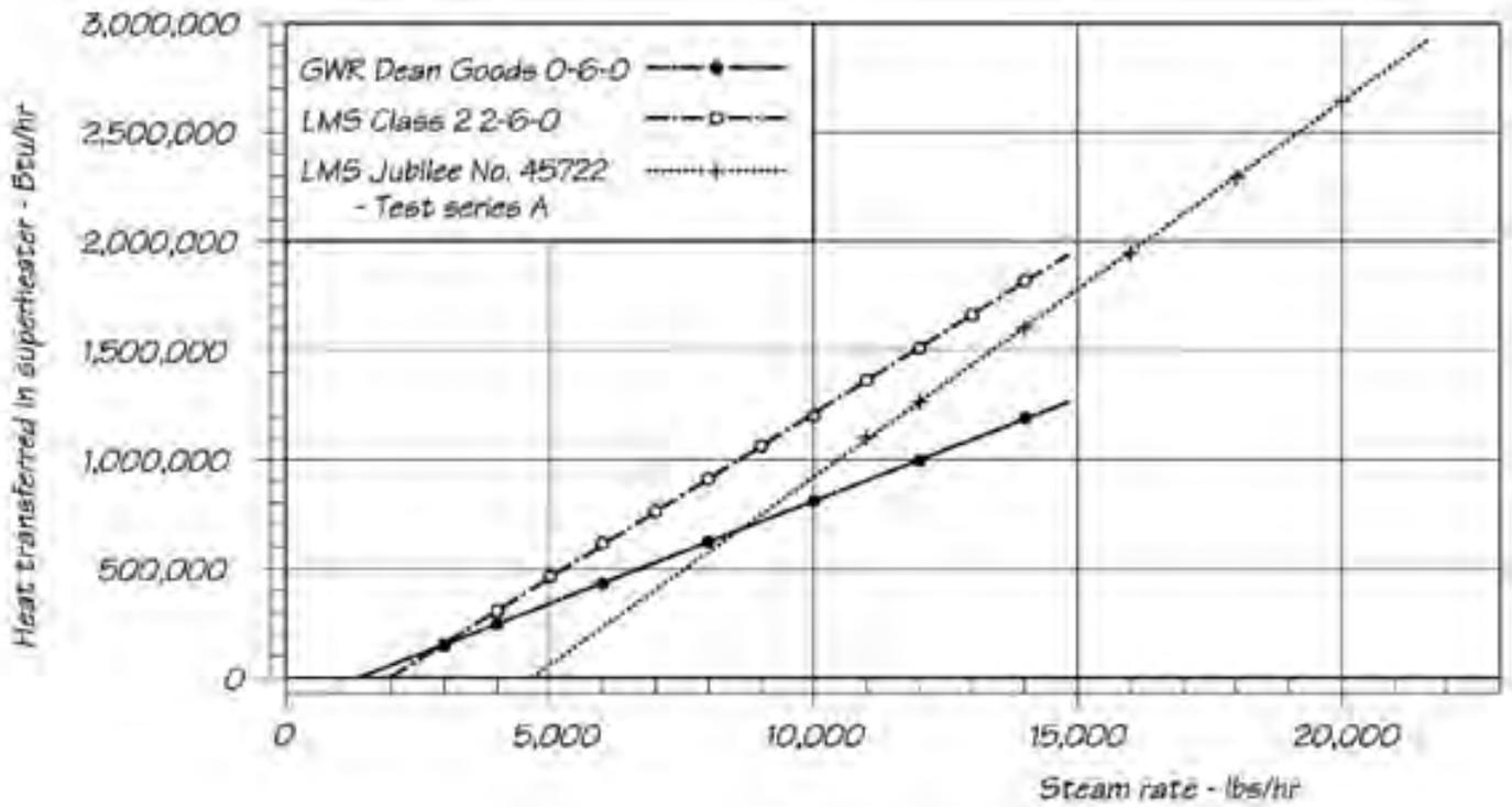
Rate of heat absorption in three superheater designs assuming a constant saturated steam inlet condition of 0.98 dryness
