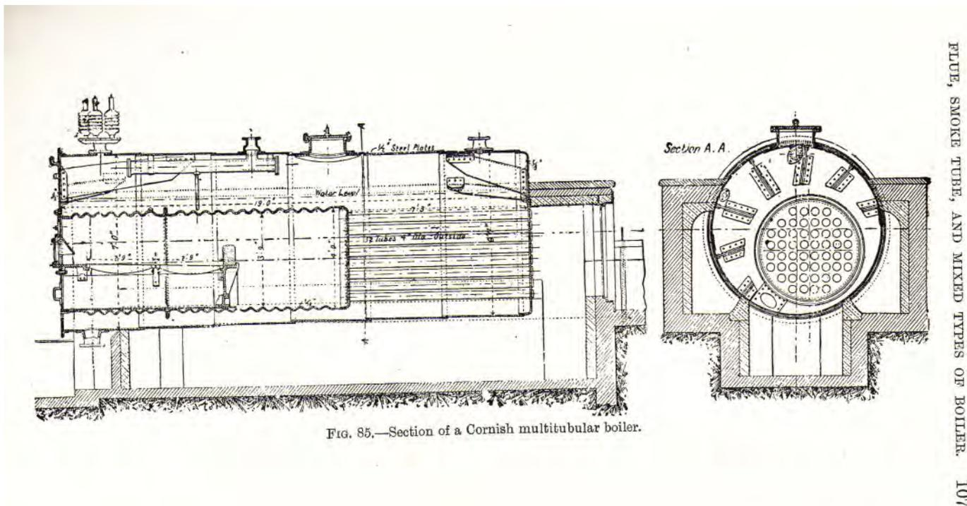
FIG. 85.—Section of a Cornish multitubular boiler.
