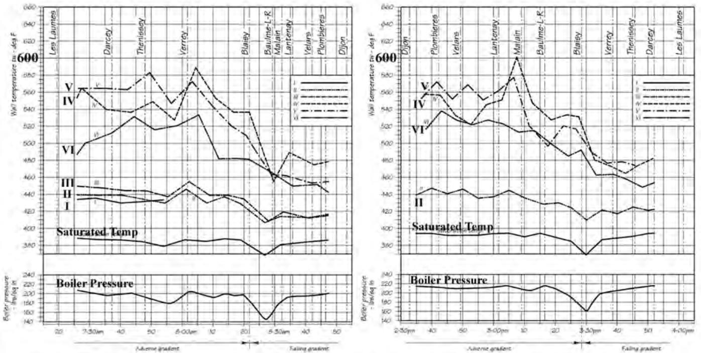
Copper firebox - locomotive No. 141-G-448; left hand diagram running from Les Laumes to Dijon hauling train M.15 (902 tons) on 29th February 1940; right hand diagram running from Dijon to Les Laumes hauling train M.52 (894 tons) on 1st March 1940.
