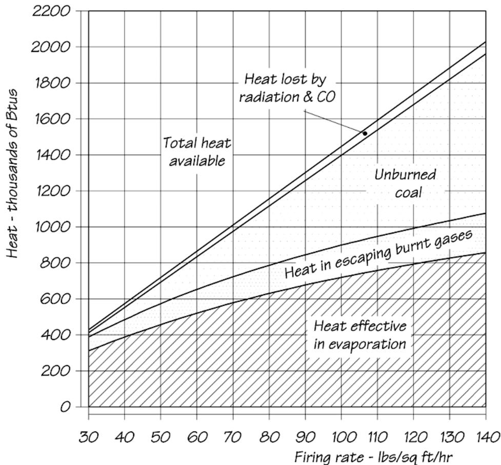
Fig. IV.10 - Approximate heat utilized and lost per square foot of grate per hour at different firing rates - St Louis Test Series 200 - Lake Shore & Michigan Southern Railway 2-8-0 N° 734
