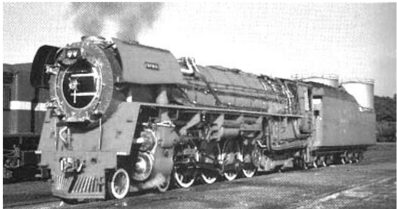
Wardale's 3,300 kW (4,500 hp) South African Railways Class 26 “Red Devil” – capable of 160 km/h performance if it had been allowed.
