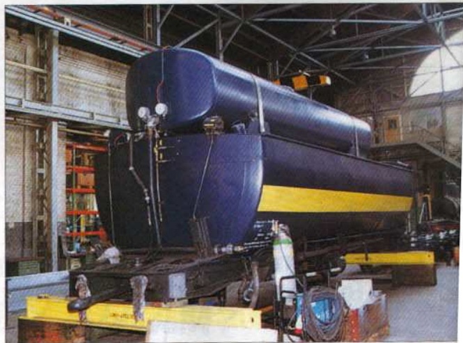
Right: Inside the main erection shop at Winterthur, where so many Swiss steam and electric locomotives have been built, is the tender for No. 52.8055 viewed from the cab end showing the oil and water capacity gauges. At the rear is the former SLM works shunter. CHRIS MILNER.
