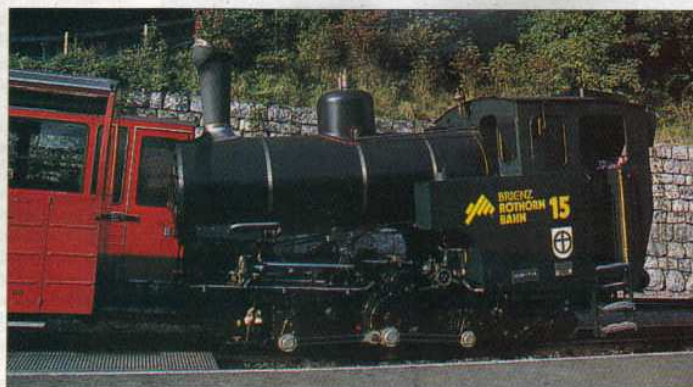
Left: A close-up of the Brienzer-Rothorn Bahn's SLM-built 0-4-2T No. 15 – which uses new steam technology – leaving Brienzer station on September 8. It's hard to believe that this loco is just three years old. CHRIS MILNER.
