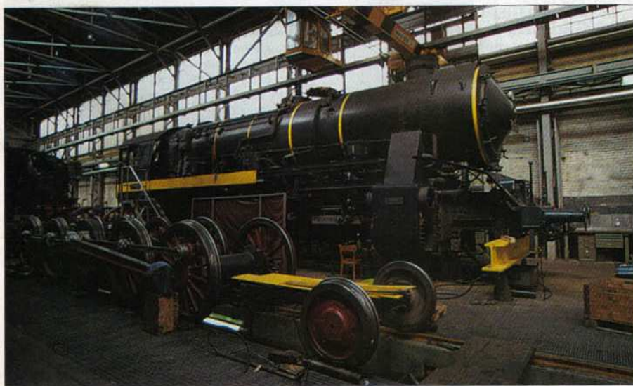
On September 7, 52.8055 was undergoing attention to its horn guides and other components at Winterthur. Despite the apparent intensity of the repairs with all wheels out, Roger Waller was confident that the loco would be back in one piece by October. CHRIS MILNER.
