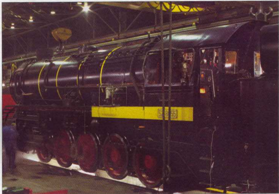
Right: Inside the main erection shop at Winterthur, where so many Swiss steam and electric locomotives have been built, is the tender for No. 52.8055 viewed from the cab end showing the oil and water capacity gauges. At the rear is the former SLM works shunter. CHRIS MILNER.
