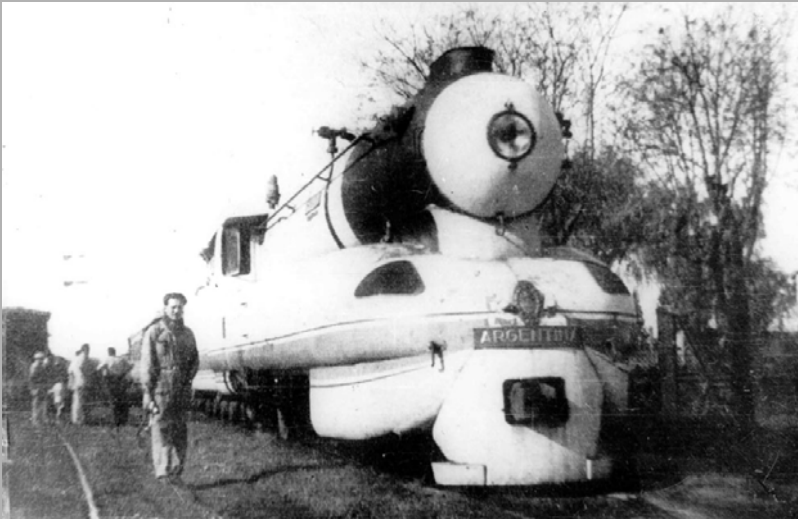
“La Argentina” by Porta 3 cylinder 4-8-0 compound Dbte 11.9%
