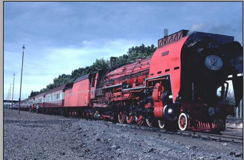
SAR Class 26 D.Wardale’s “Red Devil” 2 cylinder 4-8-4 simple Indicted te 13%
