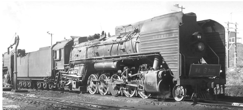
Chinese QJ standard heavy haul freight locomotive. Design dates from the 1950s.
