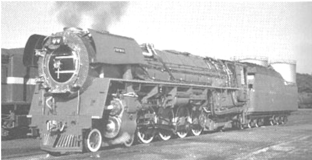
David Wardale’s “Red Devil”. A rebuild of a South African Railways Class 25NC, the locomotive’s power output was increased by 60% and its specific coal consumption was reduced by 40%.
