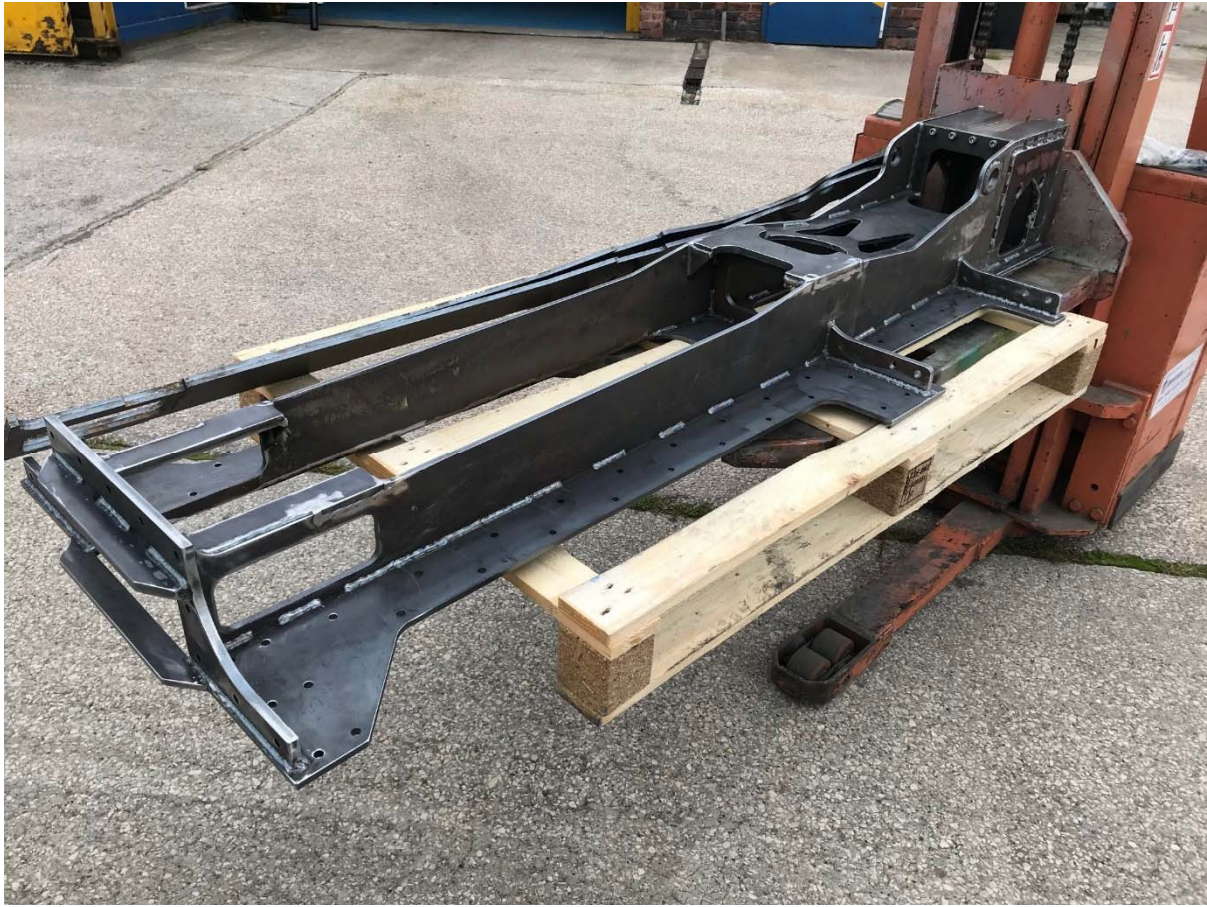
Main frame assembly (upside down)
