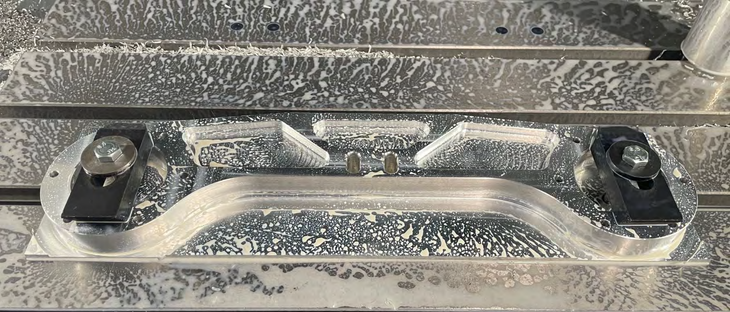
Bogie side frame –machined from solid
