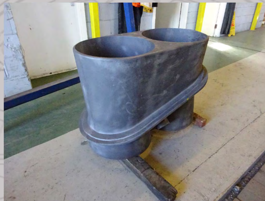
Chimney casting from Spheroidal Graphite Iron
