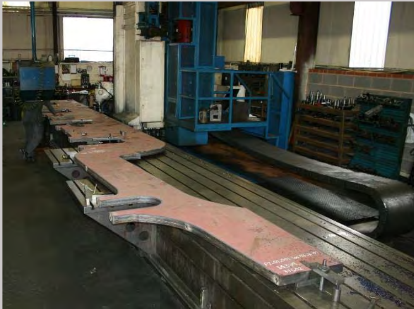
Frame plates CNC machined direct from CAD drawings by Boro' Foundry
