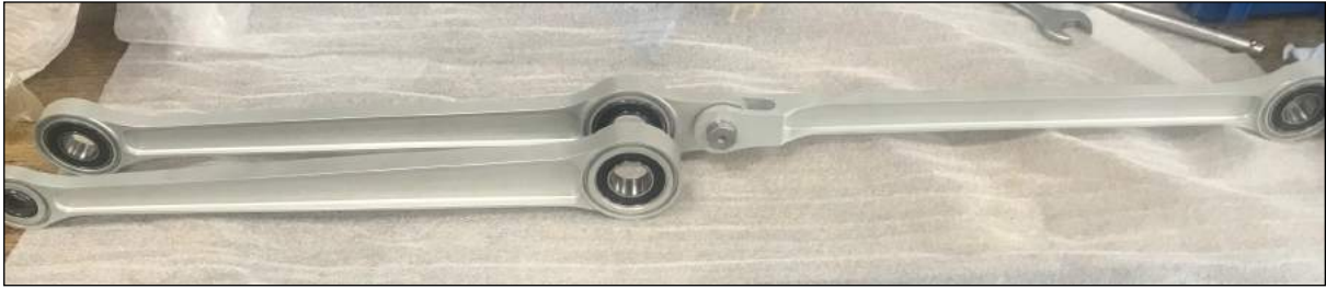
Aluminium connecting and coupling rods fitted with roller bearings
