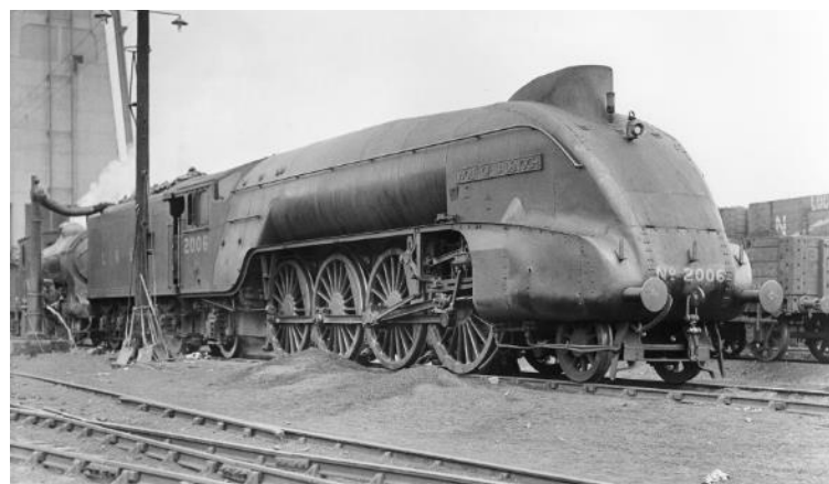
No. 2006 Wolf of Badenoch - longer combustion chamber in firebox - prototype for Tornado's boiler
