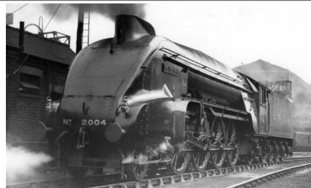
No. 2004 Mons Meg - bypass valve to divert exhaust from the blastpipe
