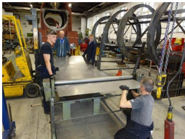
Cleveland Bridge apprentices assist with rolling cladding sheets
